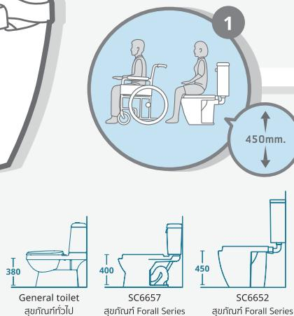
Special Height 400 mm. With SC6657 and 450 mm. With SC6652 to facilitate elder when using. (Suggestion: For elder or disable person using wheel chair have to select with 450 mm. Height for safety.)
